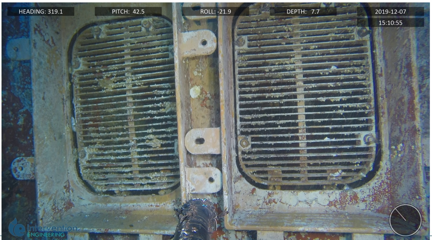
After about one hour cleaning – Some small amount of hard growth (limpets) and some antifouling coating loss (from cleaning)
