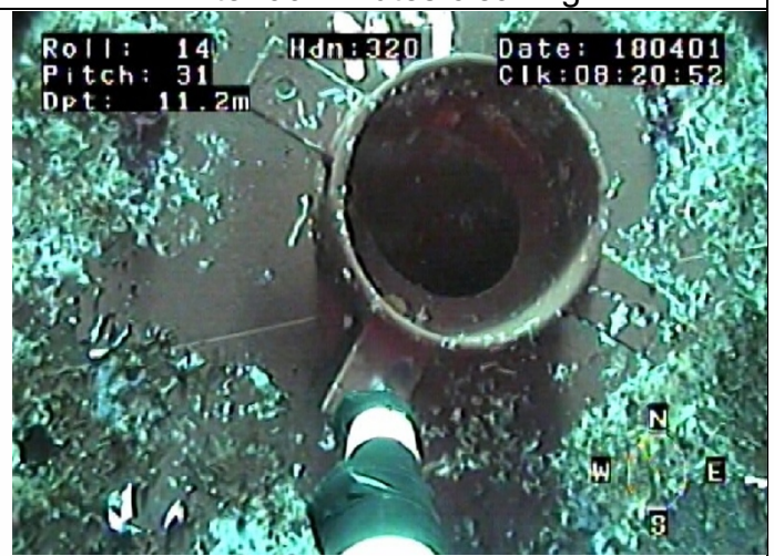
Overboard after 20 minutes cleaning
